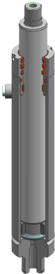
Displacement: with seal made on the rod.
